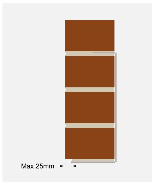
Lintels should always be propped during construction to achieve the safe working load capacities declared in the design tables in this data sheet. A separate DPC is required above the lintel. Wall ties should be installed within 300mm of the lintel at a maximum of 450mm centres to ensure that the masonry carried by the lintel is restrained and any potential overturning and deflection is minimised.
